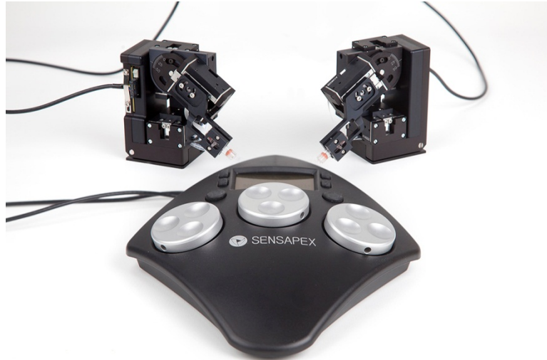
Figure 1. Photograph of a dual micromanipulator system showing the control unit and two micromanipulators with microelectrodes (left- and right-handed versions)
