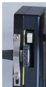
Figure 6. Micromanipulator's cable clip and power switch.
