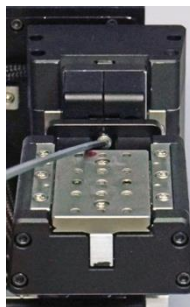
5. Attach x-axis to angle adjustment unit with two M2x3 screws
