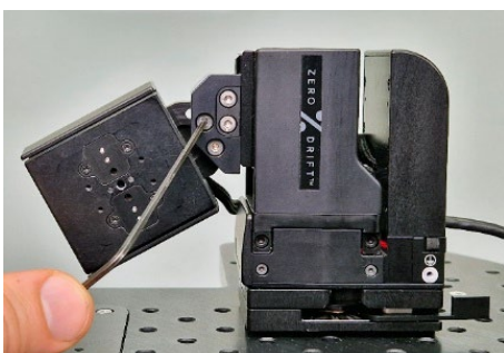
Figure 6. X / D-axis angle adjustment mechanism screws (pointed and one below it).
