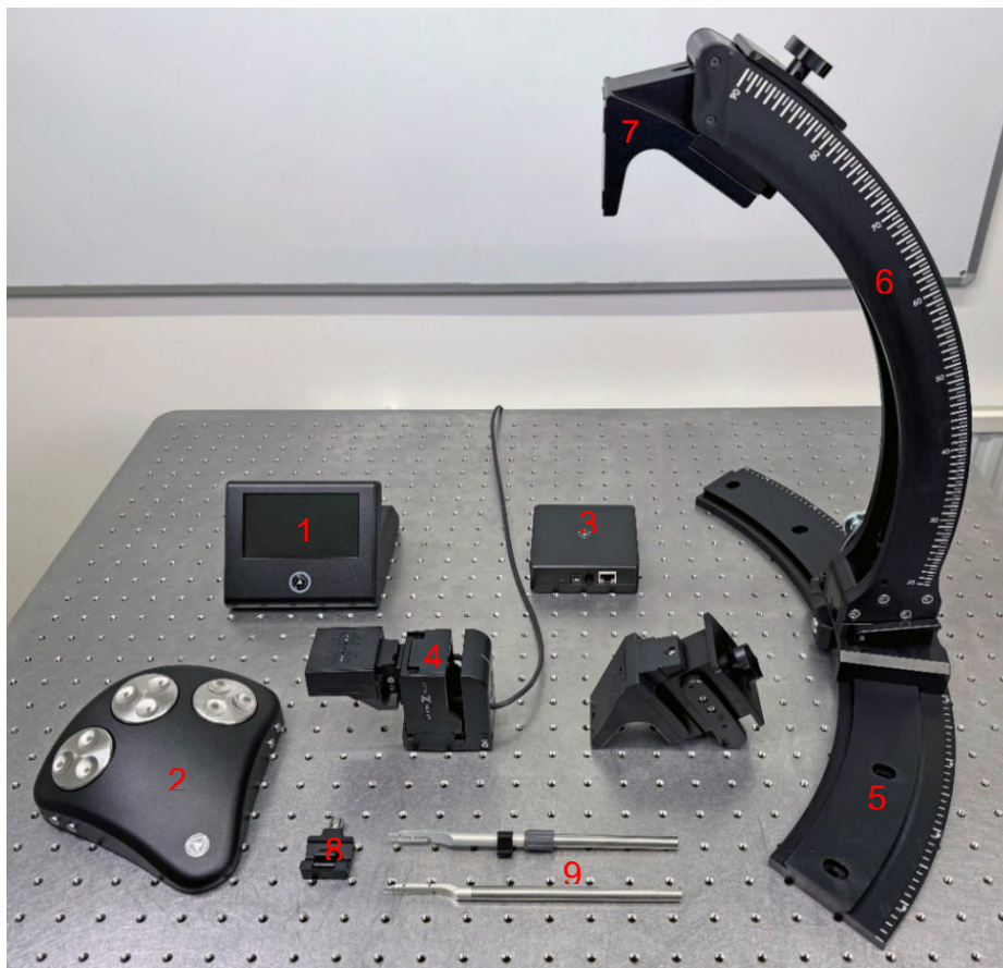
Figure 11. In vivo micromanipulator system overview
