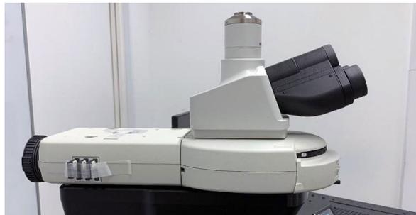
Figure 16. Installing the trinocular tube and c-mount camera adapter.
