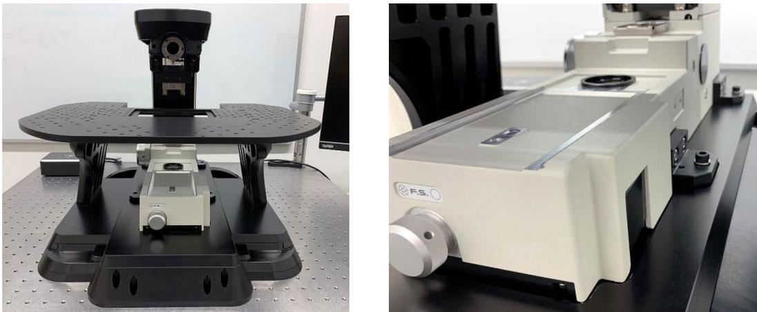
Figure 12. Installing uMs-FN1 to the uMs-BRE
