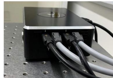
Figure 4. uMs-MXY motor and sensor cable connections.
