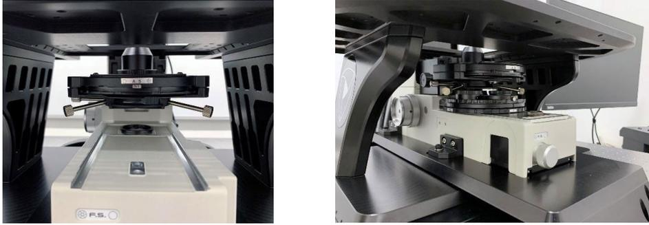
Figure 14. Left, Installing the condenser. Right, Installing the polarizer turret for DIC.
